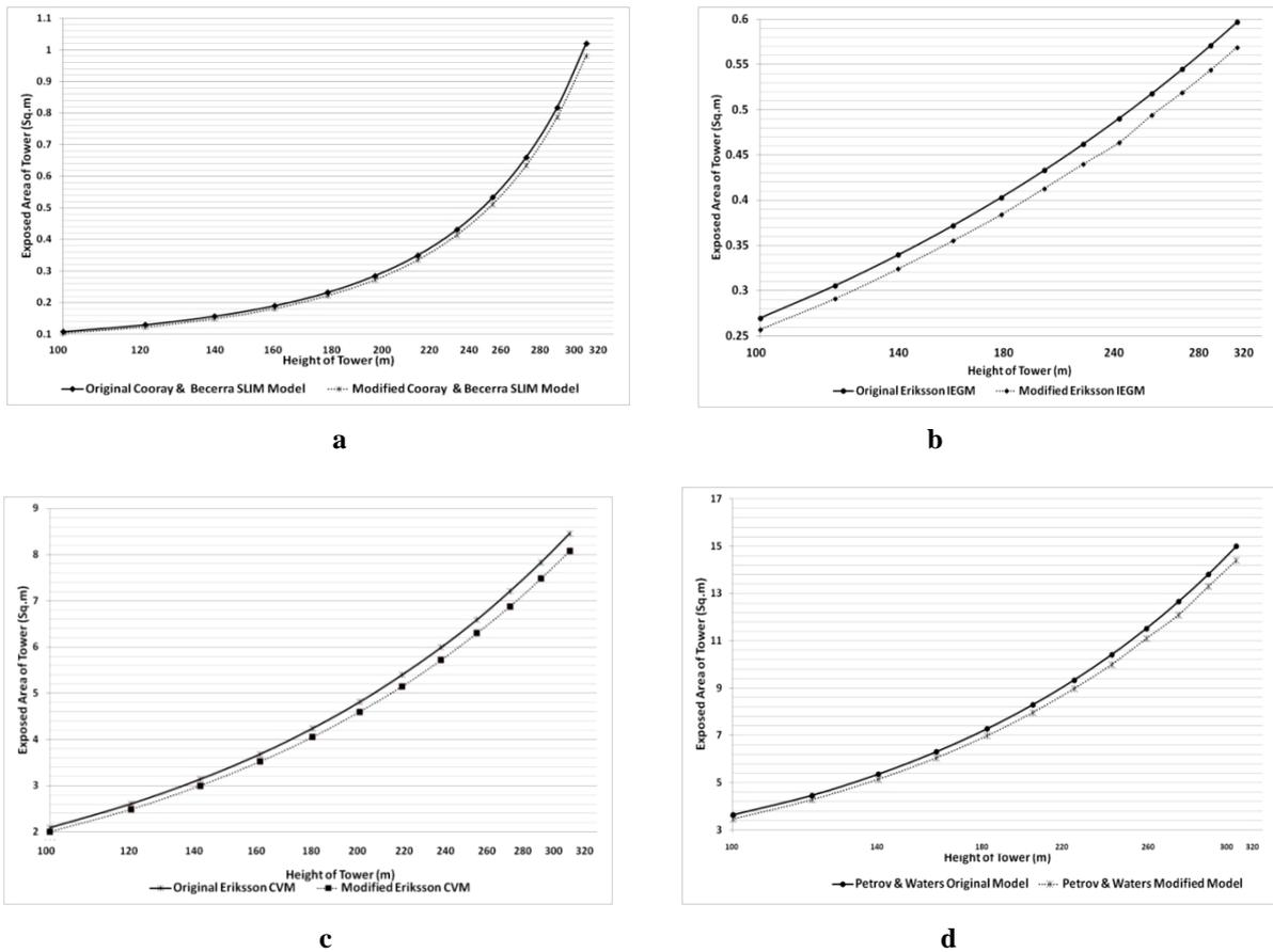
**Figure 3(a): Exposed Area of Tower of SLIM Models vs. Height of Tower; (b) Exposed Area of Tower of Eriksson IEGM Models vs. Height of Tower; (c) Exposed Area of Tower of Eriksson CVM Models vs. Height of Tower; (d) Exposed Area of Tower of Petrov & Waters CVM Models vs. Height of Tower**
